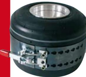
The first time you pump up the tyres after having mounted them onto the rim is most important (also for safety reasons). Use a belt around the rubber to avoid exceeding 4 bar, be very careful not to stretch the ply.
