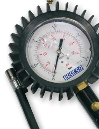
IT IS IMPORTANT TO CHECK EVERY NOW AND THEN THAT THE GAUGING IS CORRECT ANT TRUE... ALL YOU HAVE TO DO IS A PARALLEL MATCH, MEASURING THE PRESSURE OF A TYRE WITH OUR PRESSURE GAUGE AND OUR FRIEND'S PRESSURE GAUGE
